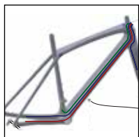
Brake/shift routing – mechanical
