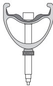
Figure 2. Place the TubeLess Ready valve through the rim strip and the rim.
