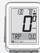
Figure 8. Ride Mode with Speed Displayed.
