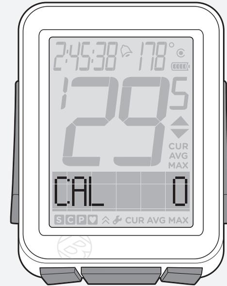
Figure 15. Calorie Output Function.
