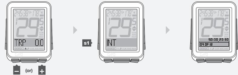
3. To restart the clock at **00:00**, hold **s1** for three seconds.
