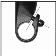
Figure 3: Clamp bolt perpendicular to radius
