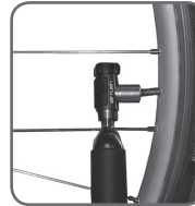
Figure 5. Inflating the tire with the cartridge in the upright position
