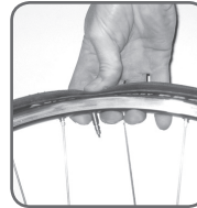
Figure 4. Squeeze the tire to extend the valve
