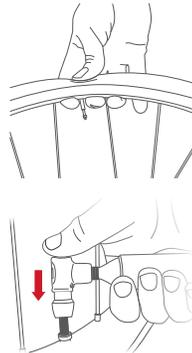
**NOTE:** Avoid inflating the tire too rapidly. Make sure the tire beads are correctly seated in the rim.
