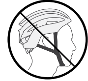
Figure 2. Incorrect helmet position
