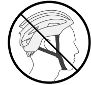
Figure 2. Incorrect helmet position
