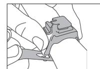
3. From the front, slide the light onto the bracket until the light engages.
