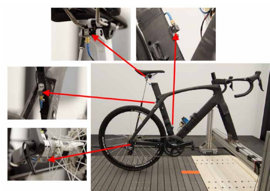
Figure A4. Triaxle accelerometer distribution.
