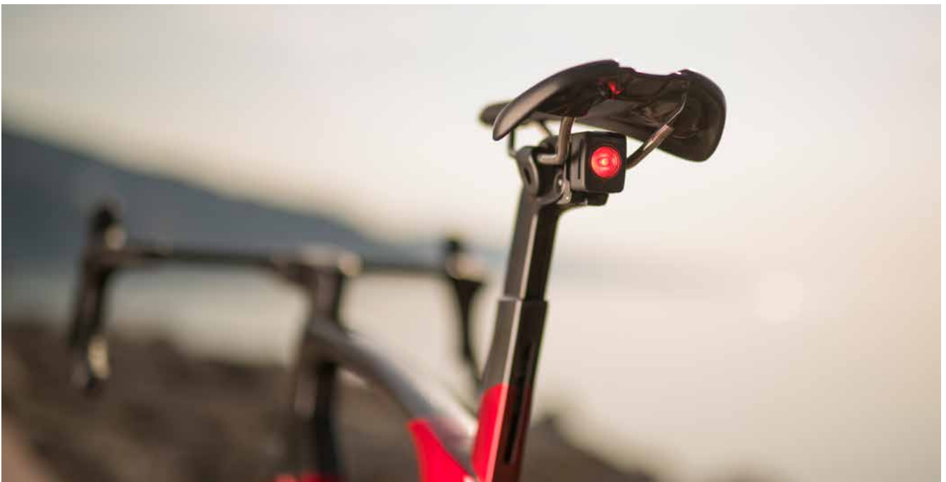
Figure 19. New Madone Seatpost with Integrated Light Mount
