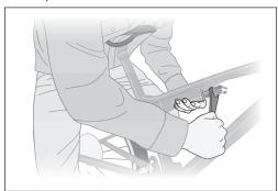
**8.** Once the ring is threaded off the shock, the forward end of the shock will extend forward to reveal an o-ring, a round metal plate, and the spacer.
