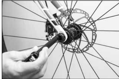
FIGURE 6 Inserting the thru-axle through the fork and hub
