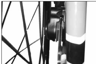
FIGURE 7 Inserting the disc
