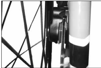
FIGURE 7 Inserting the disc
