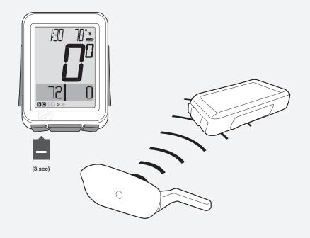
Figure 7. Icons Show Sensors are Connected.
