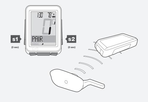
Figure 6. Locking onto Radio Signals from Sensors.
