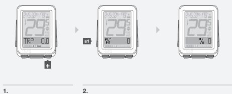
To see the gain (+) or loss (-) in Trip or Total, scroll to that feature and toggle M.
