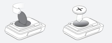
Figure 34. Removing the Battery Cover.
