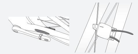
Figure 32. DuoTrap Sensor in Chainstay.
