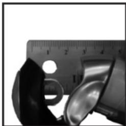
*Figure 7- Minimum lever opening*
