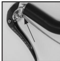
Figure 6- Cable exit hole
