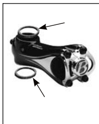
FIGURE 3.4 Required spacers above and below a direct-connect stem
