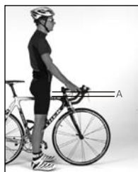
FIGURE 1.1 Minimum standover height A = 1" (25 mm) for most bicycles 2-3" (50-75 mm) for mountain bicycles
