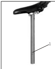
FIGURE 3.8 Minimum-insertion mark on seatpost 1. The bicycle frame should hide this line
