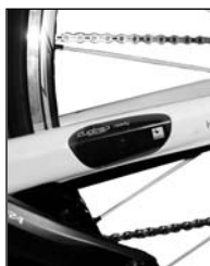
FIGURE 3.42 Duotrap integrated computer mount on chainstay for speed and cadence sensors
